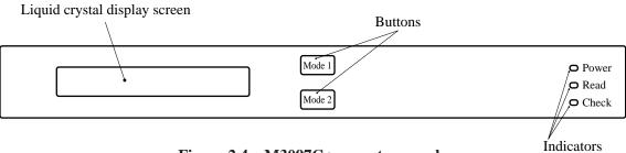
Figure 2.4 M3097G+ operator panel
